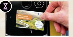
Hold the card in front of the contact sensor til the hourglass symbol disappears and the green battery symbol appears.
